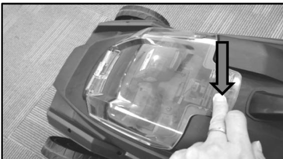
**To remove the battery cartridge from the mower:**
